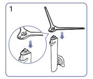
Put the stand base onto the stand neck as the direction shown in the figure. Check that the stand neck is firmly connected.
