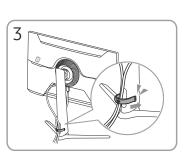
Put both cables in the cable holder on the stand (HOLDER-STAND CABLE) to organize the cables, as shown in the figure.
