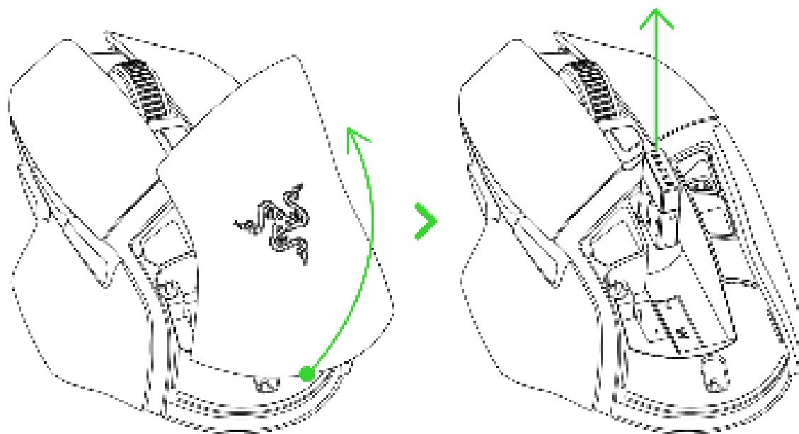
2. Reattach the top cover and plug the wireless USB dongle into your PC.
