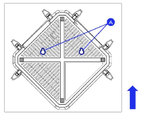
A: 2 Wall Mount Holes in blue outlines at 10cm or 4inches wide. Follow the reference image above for correct orientation and proper device mounting. Note:
