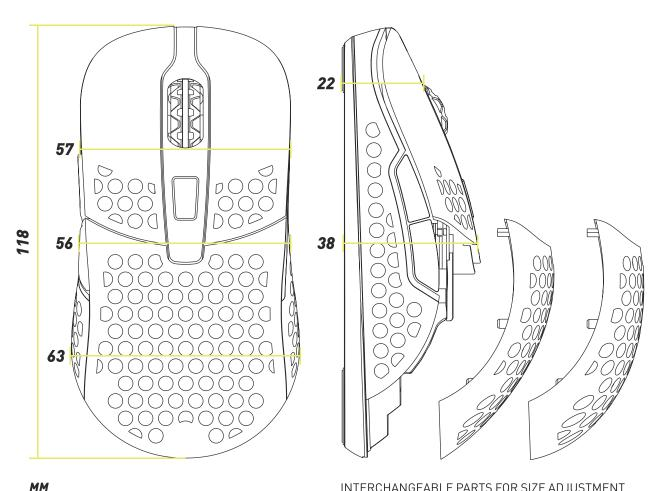
INTERCHANGEABLE PARTS FOR SIZE ADJUSTMENT
